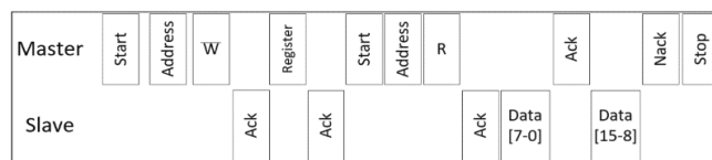
Figure R. Read Register Operation
